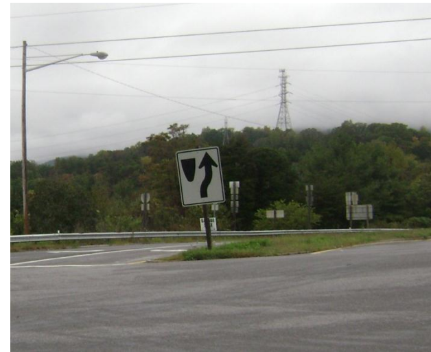
Photograph 5.6 – Keep Right Sign Mounted on North Side of Intersection – Obscures the Co-located Stop Sign
