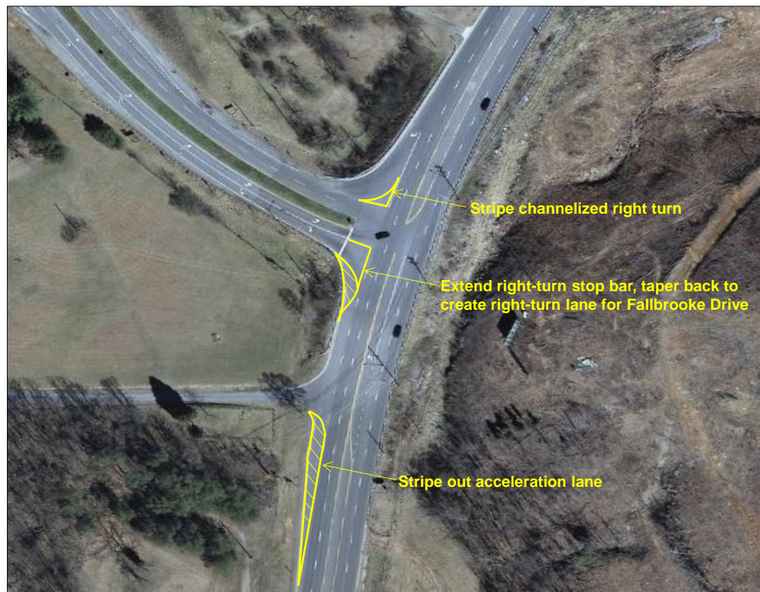
Figure 5.1 – Route 11/460 and Dow Hollow Road Intersection Striping Improvements
